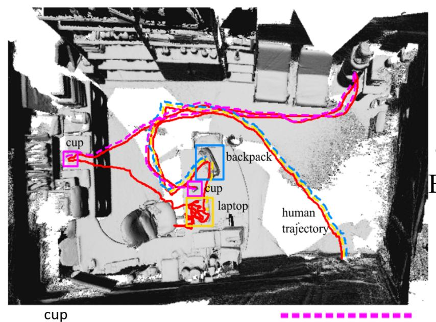
An example scenario for tracking occluded objects in an indoor scene. The dashed lines represent the inferred trajectories and different colors indicate different objects in the scene.
