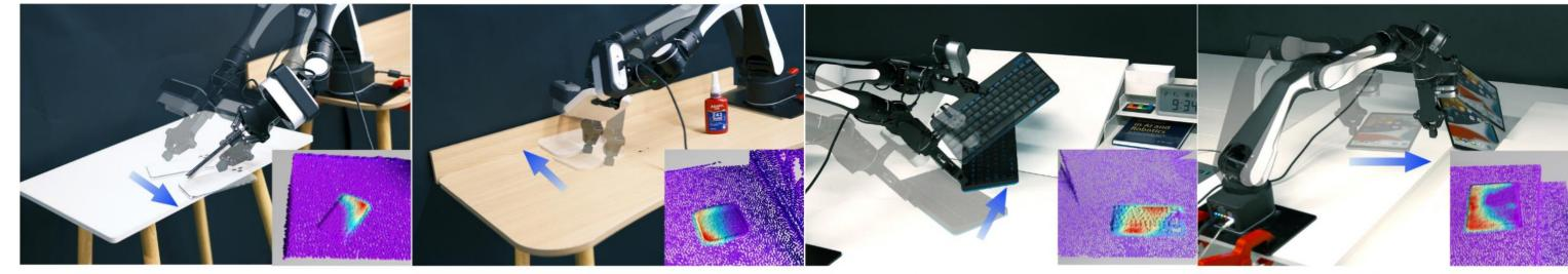
(a) move a tablet to table edge (b) push a plate towards a wall (c) push a keyboard up a slope (d) slide a tablet into a slot
