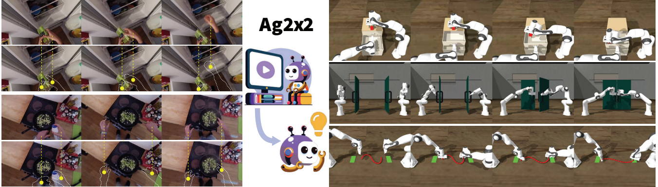
Fig. 1: Ag2x2 enables zero-shot acquisition of bimanual manipulation skills without relying on expert demonstrations or engineered rewards. The framework operates in two key stages: (left) learning coordination-aware visual representations directly from human manipulation videos (shown in sequential frames of cooking with highlighted hand) while preserving critical hand position data despite domain differences; and (right) leveraging these representations to acquire diverse bimanual manipulation skills in simulation autonomously, demonstrated through multiple Franka robot arms performing sequential steps of various tasks including cabinet opening (top row), door manipulation (middle row), and rope handling (bottom row).
