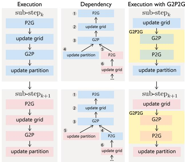
Fig. 4. **MPM pipeline reformulation.** The left column shows the traditional MPM pipeline, and the middle one illustrates an analysis of data dependencies among the sub-steps. The exchange of the *update partition* at the current time step  $k$  and the *P2G* at the next time step  $k+1$  would not break the data dependency or the execution correctness, making it possible to reorder and assemble the *G2P* and the *P2G* to form a more efficient *G2P2G* kernel, as shown on the right.
