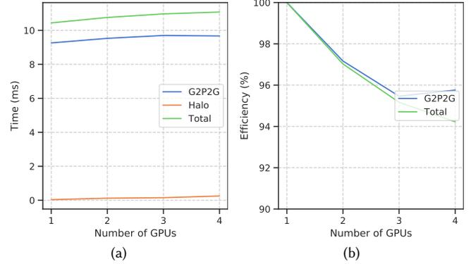
**Fig. 12. Weak scaling; compact layout.** (a) The per time-step wall time remains steady with an increasing number of GPUs for the *G2P2G* and overall performances. The additional overhead of halo tagging is growing but remains insignificant. (b) Both the *G2P2G* kernel and the overall efficiencies still stay around 95% even when employing 4 GPU devices.
