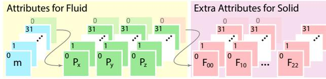
Fig. 7. **Binning.** The internal layout of each particle bin is SoA. In this example, the array length of the particle bin equals to the thread group size on the NVIDIA GPU architecture (*i.e.*, 32 for an NVIDIA GPU warp) for coalesced memory access within a bin. The number of properties is flexible according to the material; we used 4 for fluids and 13 for solids.
