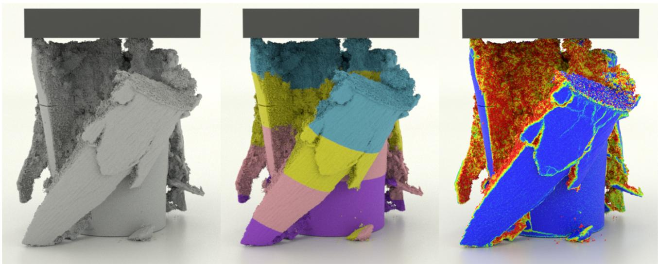
Fig. 1. **Crushing concrete.** Our system enables this concrete crushing simulation (inspired by the hydraulic press) on a single workstation with 4 NVIDIA Quadro P6000 GPUs. This simulation contains 93.8 million particles on a  $1024^3$  grid, achieving a 3.9 min/frame performance. (Left) A concrete-style render. (Middle) Coloring by GPU. (Right) Coloring by the plastic volumetric strain for visualizing the damage propagation.
