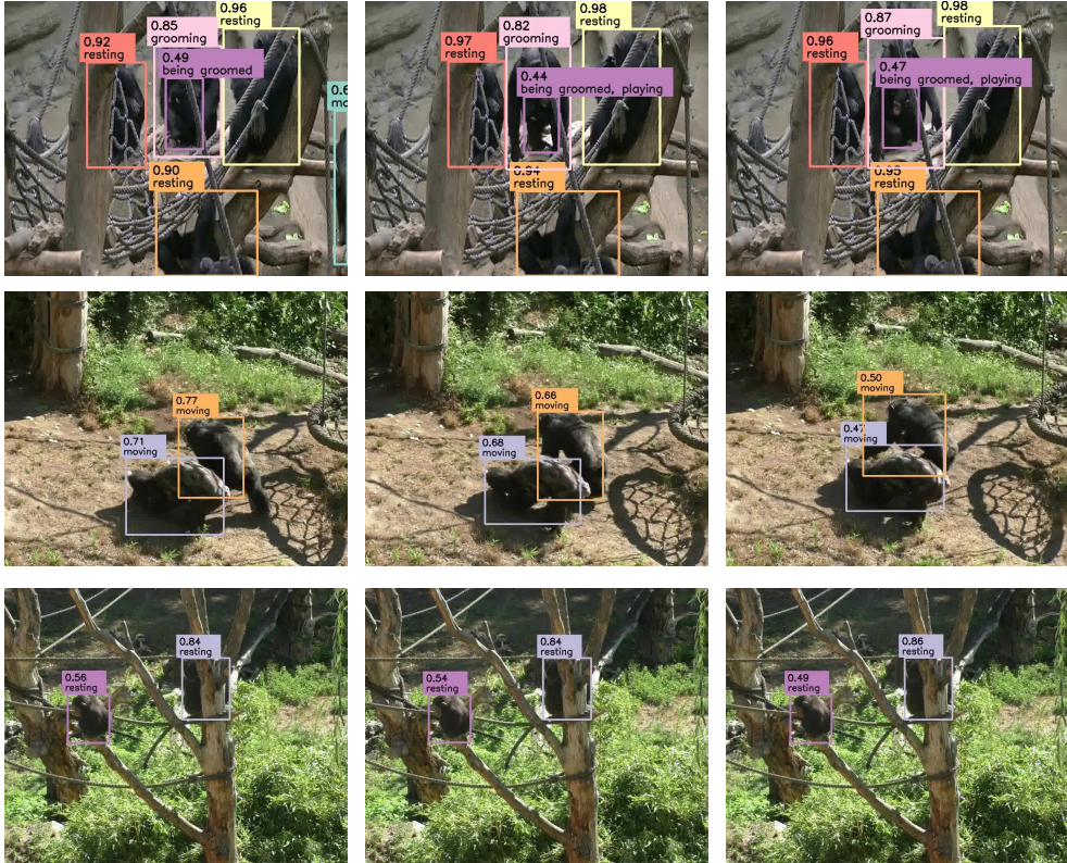
Fig. 8: Visualization of AlphaChimp’s tracking and behavior detection results in different scenarios from ChimpACT test set. Consistent colored boxes indicate successful tracking of the same chimpanzee across frames. The numbers represent the confidence scores of chimpanzee classification.
