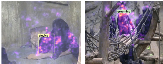
Fig. 10: Visualization of the behavior recognition probability gradient. We visualize \frac{\partial \mathbf{a}}{\partial \mathbf{I}} , where \mathbf{a} represents the behavior recognition probability for the specific chimpanzee boxed in the image \mathbf{I} .
